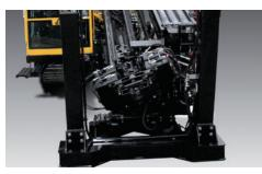
**OPEN-TOP VISE.** An angled, open-top vise allows for the passage of larger tooling. Because of the large opening, operators can also use it to break out tooling.
