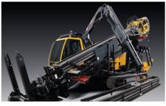
**OPTIONAL ONBOARD CRANE.** Choose the optional onboard knuckleboom style crane to reduce the amount of support equipment needed onsite.
