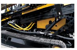
**INCREASE YOUR RANGE.** Unique four-bar linkage rack and additional pads allow operators to set up entry angles of  $11^\circ - 24^\circ$  — increasing range attainable with tracks fully on ground.
