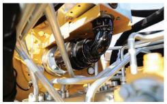
MUD FLOW. The enhanced water course system features four 1.5-in (3.8-cm) mudlines and a 3-in (7.6-cm) head shaft, allowing high volumes of fluid to be pumped downhole.
