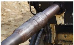
DRILL ROD ADVANTAGES. Outfitting the drill with a 30-ft (9.1-m) rack gives crews the ability to use a variety of range 2 drill pipe, helping decrease the number of tool joint connections – the optimal setup for performing pipeline work.
