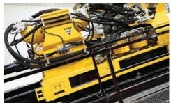
POWERFUL TORQUE. Operators can adjust the drill from 30,000 ft-lb to 52,600 ft-lb (40,675 Nm to 71,316.1 Nm) of rotary torque, with max torque being highly advantageous when turning large-diameter reamers and hole openers for installing large-diameter product.
